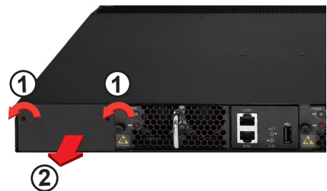
Figure 3-1: Removing the Blank Plate
