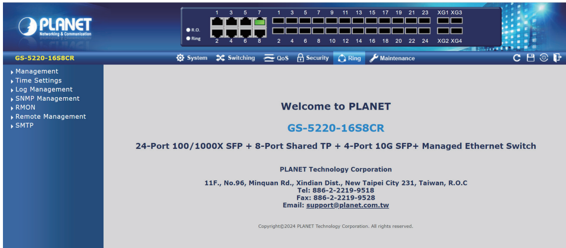
Figure 5-4: Web Main Screen of Managed Switch
