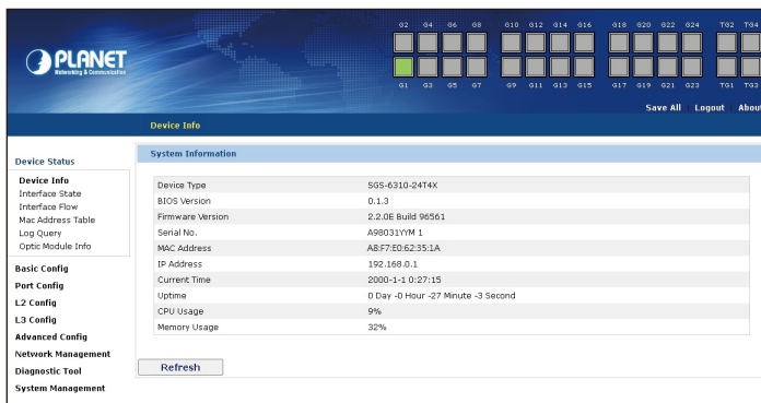
Figure 5-3: Web Main Screen of Managed Switch
