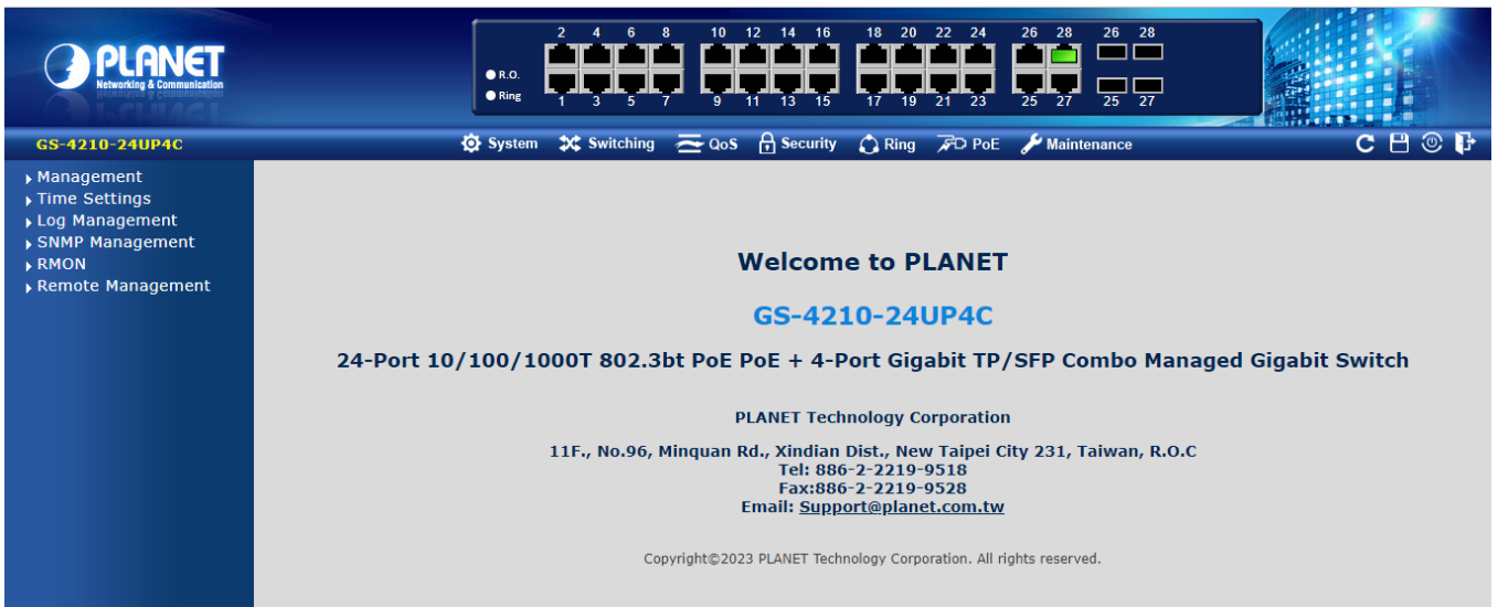
Figure 3-1-4 Web Main Screen of Managed Switch
