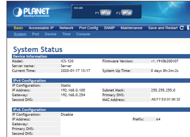
Figure 4-3: Web Main Screen of Serial Device Server
