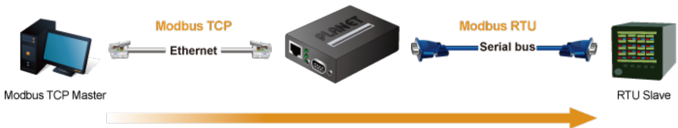
Figure 4-5-5: RTU Slave Topology
