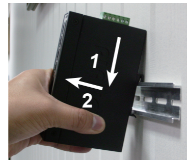
Figure 5-3: Removal of Device from Track
