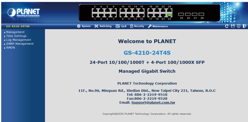
Figure 4-3: Web Main Screen of Managed Switch
